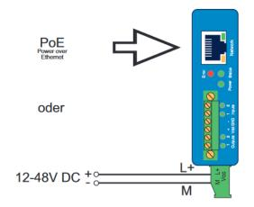
Figure 3 Supply voltage connection
