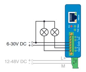
Figure 4 Output wiring
