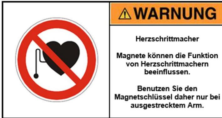
For people or residents with a pacemaker, make sure that a safety distance of at least 0.5 m between the magnetic key and the pacemaker is maintained. It is recommended to remove the transponder with an outstretched arm, as the function of pacemakers can be influenced by magnets.
